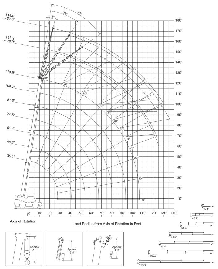
NOTE: Boom and jib geometry shown are for unloaded condition and machine standing level on firm supporting surface. Boom deflection and subsequent radius and boom angle change must be accounted for when applying load to hook.
